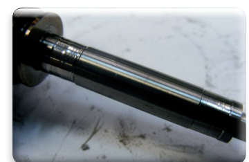
Extreme wear on the turbine shaft
