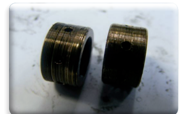
Severe scoring on to the journal bearings
