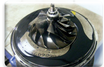
Compressor end oil leakage due to low air pressure
