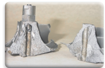
Compressor destroyed by overspeeding
