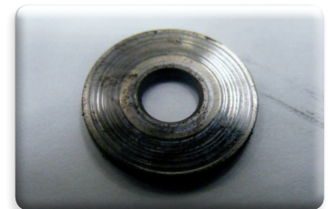
This marking is evidence of contaminated oil
