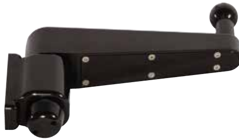
DA8861 Billet Wing Mirror Arms Defender - all models Black. Supplied as a pair. Manufactured from aerospace grade billet aluminium, anodised and assembled in house at Optimill. Designed to fit both original and Optimill door hinges. All fixings and drilling templates are supplied for ease of fitting. These arms are 20mm longer to aid towing trailers/caravans.
