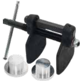
Brake Caliper Rebuild Tool Kit DA1153 After a brake caliper rebuild the most difficult part can be fitting the dust seal after the pistons have been fitted. Make that task easier with the seal fitting tools in this kit. The kit is supplied with a tool to fit 41mm and 44mm pistons and comes complete with a heavy-duty piston spreader to allow the seals to be pushed into place evenly. DA7460 Heavy-duty piston spreader only.
