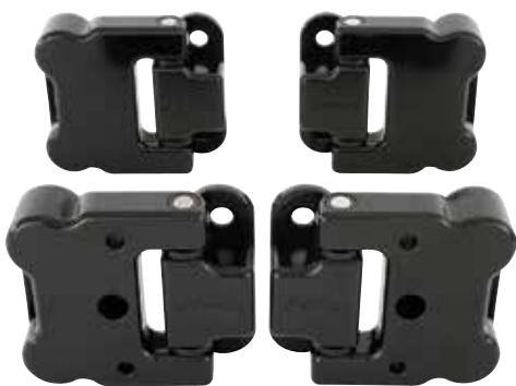
DA8864 Front Door Security Hinge Kit Defender 90 - all models Black With this unique design the door cannot be removed even if the external screws have been removed. Prevention increases security for unwanted removal. These high quality door hinges are CNC machined from billets of aerospace grade 6082-T6 aluminium. The hinge pins are made of stainless steel which are internally pinned to prevent unwanted removal or theft. The hinges also feature self lubricating graphite bushes to reduce friction and prevent wear. Supplied with high security stainless fixings & shims.
