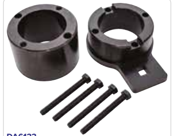
DA6133 Crankshaft Pulley Holding Tool Provides the required components to hold the crankshaft vibration damper in place whilst undoing the very tight pulley mounting bolt. Equivalent to OEM 303-191, 303-192, 303-193, 303-194. Designed to be used with a 1/2" D Power Bar. For use on AJ V8 3.2, 4.0, 4.2 & 4.4 petrol engines.
