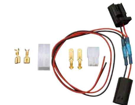
DA8862LOOM Wiring Loom For Number Plate Light With Reversing Camera Small piggy back wiring loom that fits between original plug and reversing light, enabling fitment of the new number plate light and provide the live power feed for the reversing camera.
