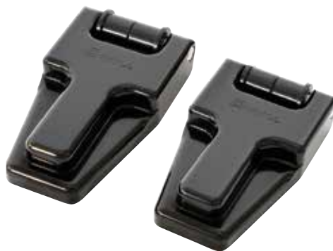
DA8867 Security Bonnet Hinge Kit Defender - all models Black. Supplied as a pair. These are CNC machined billets of aluminium 6082-T6. Internally pinned to prevent unwanted removal of the bonnet. Anodised for extra protection and longevity. The set comprises of high security stainless steel fixings which are fixed from underneath the bonnet for added security.
