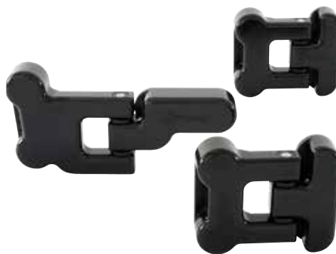
DA8867 Security Bonnet Hinge Kit Defender - all models Black. Supplied as a pair. These are CNC machined billets of aluminium 6082-T6. Internally pinned to prevent unwanted removal of the bonnet. Anodised for extra protection and longevity. The set comprises of high security stainless steel fixings which are fixed from underneath the bonnet for added security.
