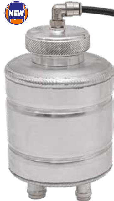
DA4749 NEW Aluminium Power Steering Reservoir with Internal Baffle Defender - Tdi, Td5, Tdci & V8 Designed to replace the plastic ZF reservoir which is prone to splitting and leaking vapour through the breathable cap, which in turn then collects dirt and runs the risk of water ingress. The external breather design means no unsightly mess under the bonnet and allows routing with high axle/gearbox breathers to eliminate water ingress. Manufactured from laser cut 2mm high grade aluminium with CNC machined pipe connections, knurled cap and external breather. The corrosion resistant aluminium rolled body is fully TIG welded by hand in house. 110mm high (155mm height including cap) & 91mm diameter.
