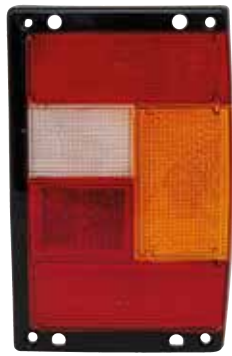
Rear light lens assembly with black border Range Rover Classic RTC4590LUCAS Right hand side RTC4591LUCAS Left hand side
