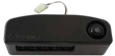
DA8862 Number Plate Light with Camera Defender - all models Black Complete with HD 170 degree camera & LED number plate light. Billet machined from 6082 aluminium. Plug & Play to plug into factory Land Rover wiring loom. Fitted using the existing holes in the body. Supplied with foam gasket and stainless steel screws.
