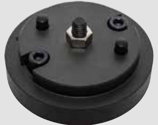
DA6550 Crankshaft Trigger Wheel Installer Tool Discovery 3/Discovery 4 Range Rover Sport - Mk1 Required to install the crankshaft position sensor ring when fitted with TdV6 engine. Specifically required to repair sensor wheel dropping off or cracking. Equivalent to OEM 303-1130 Overall dimension: 123.5mm
