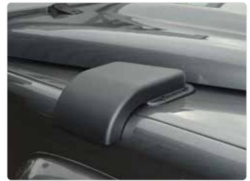
Snow Cowls Manufactured from ABS plastic these cowls will help prevent snow, mud and leaves from entering the heater intake and reducing the Defender heater performance. Fitting a cowl will reduce moisture build-up in the intake system which can happen if debris collects in the one-way valve. The cowl fits over the existing grille and follows the profile of the Defender's wing. DA1270 Left hand drive DA1271 Right hand drive
