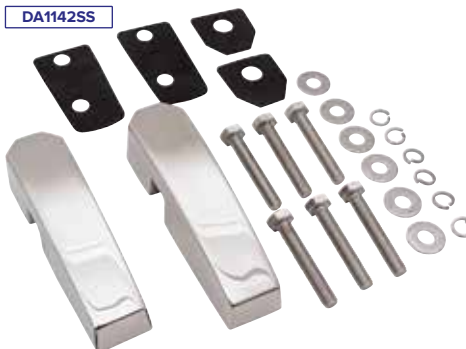
Windscreen Brackets Supplied in pairs Anodised Finish Replace your corroded Defender windscreen brackets with a pair of these smart CNC machined aluminium billet brackets which won't tarnish like the standard brackets. Kits include gaskets and bolts. For fitment to vehicles with hinge type windscreen 2 x reinforcement strap LR016671 are required.
