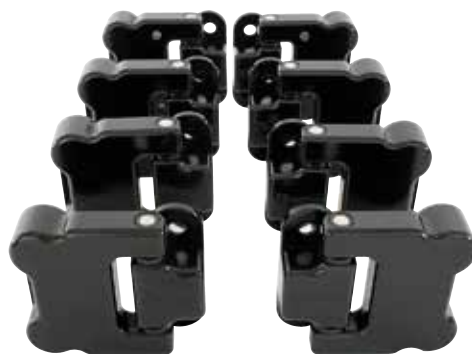
DA8864 Front Door Security Hinge Kit Defender 90 - all models Black With this unique design the door cannot be removed even if the external screws have been removed. Prevention increases security for unwanted removal. These high quality door hinges are CNC machined from billets of aerospace grade 6082-T6 aluminium. The hinge pins are made of stainless steel which are internally pinned to prevent unwanted removal or theft. The hinges also feature self lubricating graphite bushes to reduce friction and prevent wear. Supplied with high security stainless fixings & shims.
