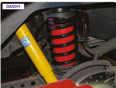
Air Lift 1000 DA5010 Defender 110/130 DA5011 Defender 90/Discovery 1/Range Rover Classic Air adjustability is the difference! Stiff steel factory suspensions must compromise between ride comfort and load hauling capacity. Smooth ride suspensions can't carry heavy loads; heavy springs ride rough, especially when the vehicle is unloaded. Air Lift adjustable air springs solve these problems by allowing you to tune your suspension under all load and road conditions. Just add air when towing or hauling and then remove air for a softer ride when unloaded.
