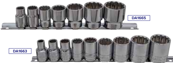
Whitworth socket sets. Manufactured from Chrome Vanadium. Complete with socket rail. DA1665 DA1663 Socket Set - Whitworth 1/2" Drive 9 Whitworth sockets in bi-hex format with 1/2" drive. Sizes - 1/8" / 3/16" / 1/4" / 5/16" / 3/8" / 7/16" / 1/2" / 9/16" / 5/8" DA1665 Socket Set - Whitworth 3/8" Drive 7 Whitworth sockets with 3/8" drive. Sizes - 1/8" / 3/16" / 1/4" / 5/16" / 3/8" / 7/16" / 1/2"
